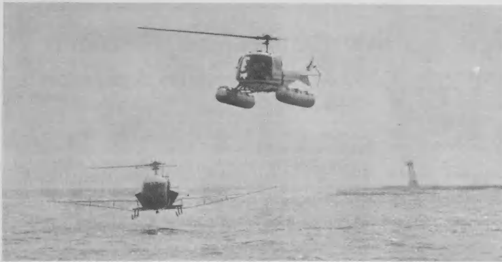
One helicopter skims sea surface to spray Corexit on oil slick while cameraman in other helicopter films action.
